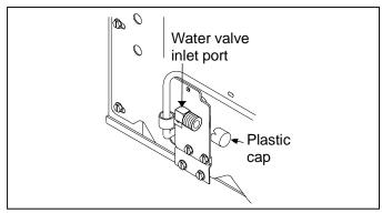
2. Place brass nut and brass sleeve on copper tubing. (Brass nut and sleeve are found in literature packet.) Insert copper tubing into water valve inlet port. Connect brass nut on copper tubing to water valve inlet port. Start connection by hand then use a 1/2" (13 mm) open end wrench. Make sure copper tubing is secure by pulling on copper tubing.
